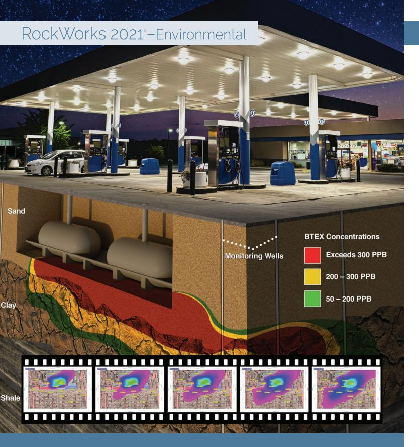
Borehole logs, cross sections, concentration maps, plume models, geology models, time-based animations, geochemistry diagrams and more. RockWorks will help the environmental professional along the path from site characterization to remediation planning and execution.
