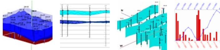
*Color Models and Diagrams:* Display color blocks in **2D** and **3D logs**. Interpolate a **solid model** for colors, display as 2D **profile slices**, **cross sections**, **projected cross sections**, **plan slices**, and as 3D **fence panels** and **voxel displays**. Determine colors from raster logs, **descriptions** or **Munsell codes**.
